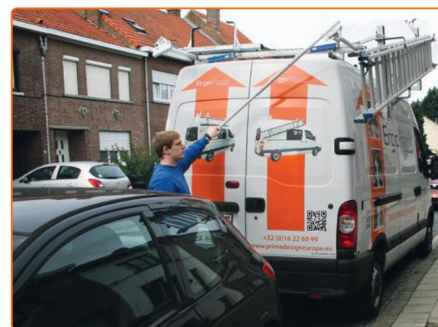
Handling from the sides makes (un)loading of ladders possible in confined parking spaces
