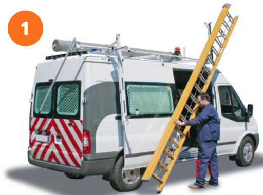
1 - Put the ladder on the front support;
